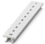
Zack marker strip, Strip, white, labeled, can be labeled with: CMS-P1-PLOTTER, Printed vertically: consecutive numbers 1 ... 10, 11 ... 20, etc. up to 491 ... 500, mounting type: snap into tall marker groove, for terminal block width: 6.2 mm, lettering field size: 6.15 x 10.5 mm, Number of individual labels: 10
