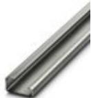
DIN rail, unperforated, G profile, width: 32 mm, height: 15 mm, acc. to EN 60715, material: Steel, galvanized, passivated with a thick layer, length: 2000 mm, color: silver
