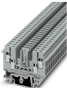
Disconnect terminal block, nom. voltage: 400 V, nominal current: 16 A, connection method: Screw connection, cross section: 0.2 mm<sup>2</sup> - 6 mm<sup>2</sup>, AWG: 24 - 10, length: 63.5 mm, width: 6.2 mm, color: gray, mounting: NS 35/7,5, NS 35/15, NS 32
