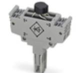
Component plug, with bridge rectifier B 250 C 1500, for 4-pos. components, reverse voltage: 600 V, nominal voltage: 250 V, nominal current: 1.5 A, two basic terminal blocks are required per plug, height: 19 mm, color: gray
